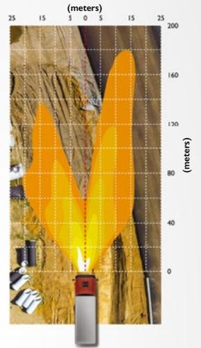
**Off-road illumination.** To ensure optimum visibility when working with your headlamps on, your headlamps need to be positioned correctly such as to provide an intense and precise source of luminous power – this is the only way to guarantee your comfort and safety while also taking the stress out of driving.
